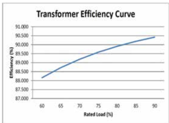
Figure 6: Transformer efficiency curve at different loads.
